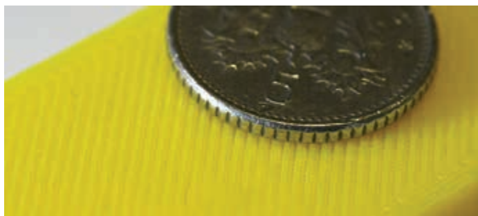
PHOTO 2: Surfaces of 3D printed objects often have a characteristic 'roughness' that can act like a grip.
