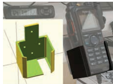
PHOTO 1: Part of a simple 3D printed project: a holder for a hand-held radio. The 3D model is on the left and the finished item in use on the right.
